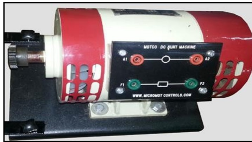
Fig. 3.3: Indigenously developed DC generator
