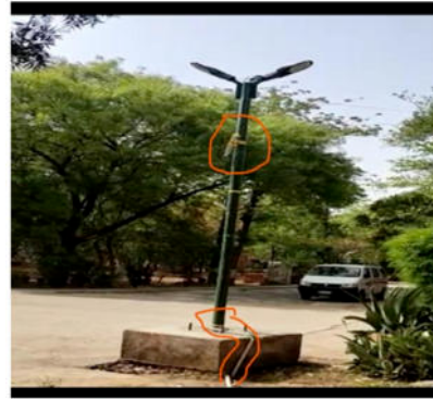
Fig. 4.5: Developed Prototype is installed at this pole of Sithauli Campus at ITM University, Gwalior, India. Initially Street Lights are in OFF Condition as the car is stationary object in this picture.
