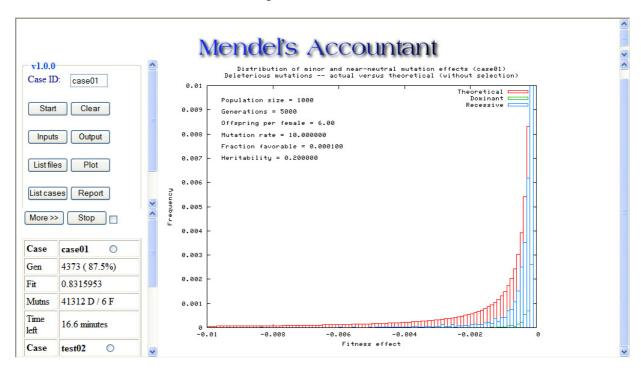
FIG. 2.4. Web user interface of Mendel's Accountant showing distribution of mutations with respect to fitness effect. Red bars represent mutation distribution in the absence of selection. Blue and green bars represent actual accumulated recessive and dominant mutations, respectively, in the presence of selection. The two bars representing mutation classes with effects nearest zero extend beyond the vertical scale of the plot.
