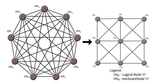
Fig. 4.2. Mapping hardware nodes of the cluster to logical nodes in the abstracted layer.
