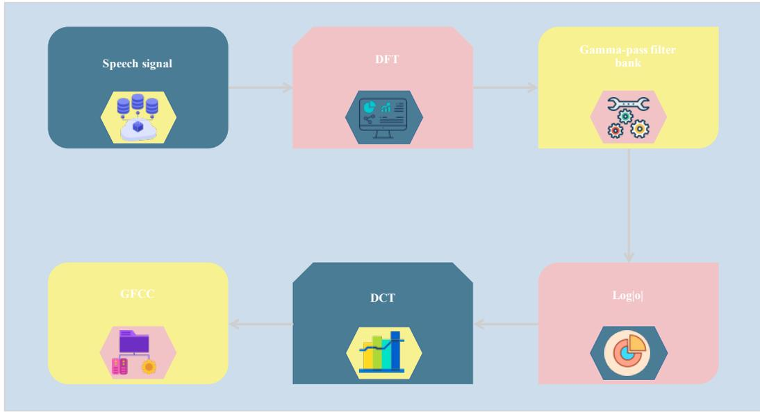
Fig. 2.1: Gammatone filter cepstrum coefficient extraction process
