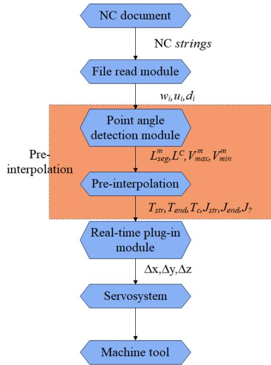
Fig. 2.1: Real-time MATLAB interpolation algorithm with look-ahead
