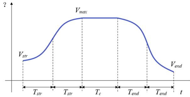
Fig. 2.9: Acc-cv-DEC acceleration and deceleration diagram
