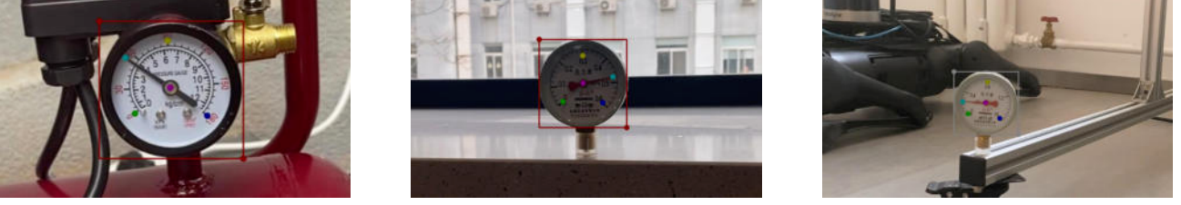
Fig. 3.1: Examples of pointer meter annotations. (a) Instrument A with a maximum range of 180 Lb/in 2 ; (b) Instrument B with a maximum range of 0.6 MPa; (c) Instrument C with a maximum range of 1.6 MPa.
