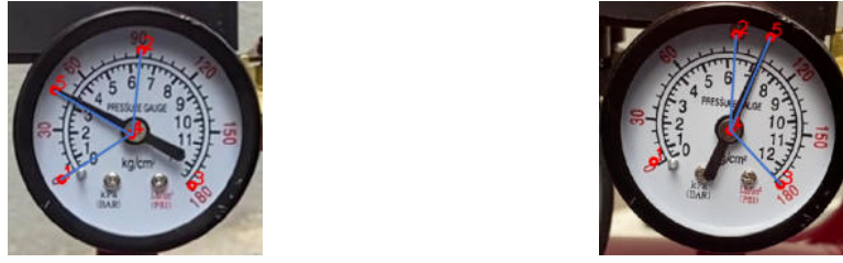
Fig. 2.5: Reading calculation methods in two cases: (a) The pointer is in the first half of the range; (b) The pointer is in the second half of the range.
