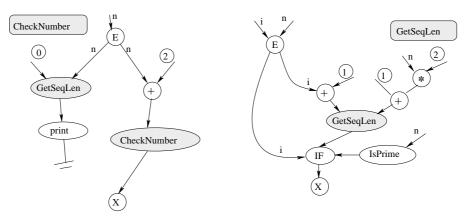
FIG. 8.1. A graph to print the length of sequences of primes generated by taking a prime, doubling it and adding one e.g., 89, 179, 359, 719. The graph is simplified for brevity; isPrime represents an invocation of isProbablePrime on the BigInteger N. \* and + correspond to the methods multiply and add. The shaded nodes represent Condensed Graph nodes
