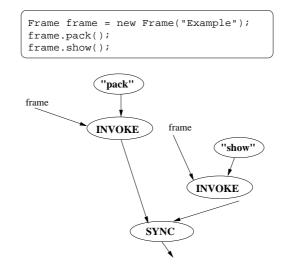
FIG. 6.8. Forcing sequential execution
