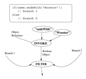
FIG. 6.3. Graph for If-Else statement using Filter node
