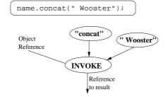
FIG. 6.2. Graph for invocation of a method on an object
