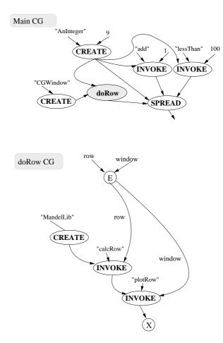
FIG. 8.2. Example program snippet to calculate and display the Mandelbrot Set converted to an automatically parallel CG The shaded nodes represent Condensed Graph nodes
