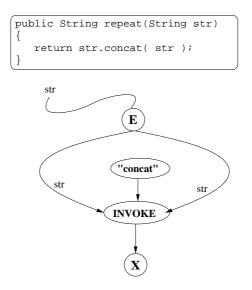
FIG. 6.5. Corresponding Graph for Methods
