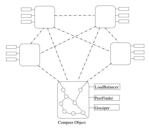
FIG. 2.1. The Competer Architecture. A system of 5 peers is illustrated with CGs running on each peer and communicating with each other. The Competer object on each peer is responsible for gathering system information, for creating objects corresponding to incoming CGs and for initiating the creation of CGs on other peers.
