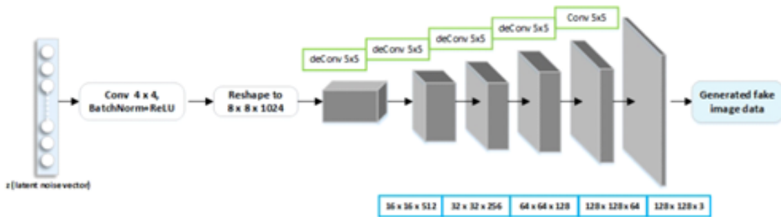
Fig. 3.3: Generator Model Architecture
