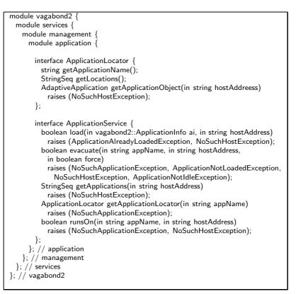
FIG. 4.2. The Application Module of Vagabond2
