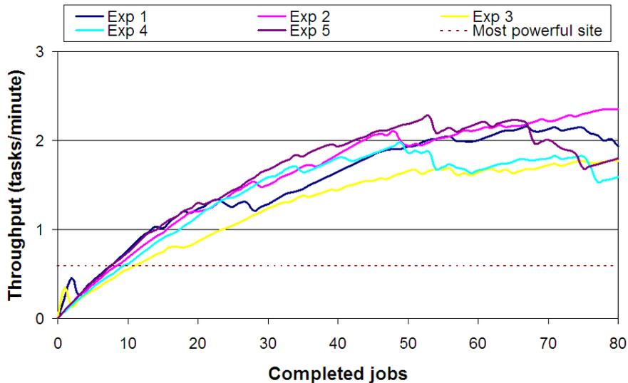
FIG. 6.1. Testbed dynamic throughput during the five experiments and theoretical throughput of the most powerful site.
