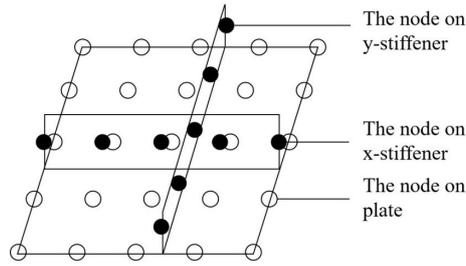
Fig. 3.1: Mesh free model with ribbed plates
