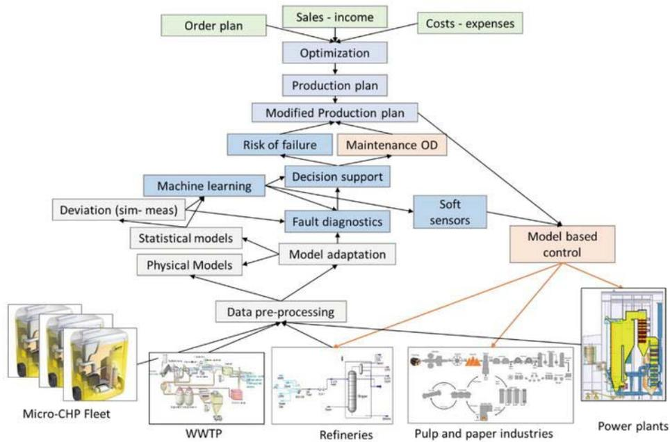
Fig. 2.3: Adaptive perception model based on artificial intelligence.
