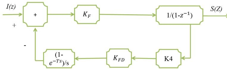
Fig. 3.6: Simplified signal transmission flowchart
