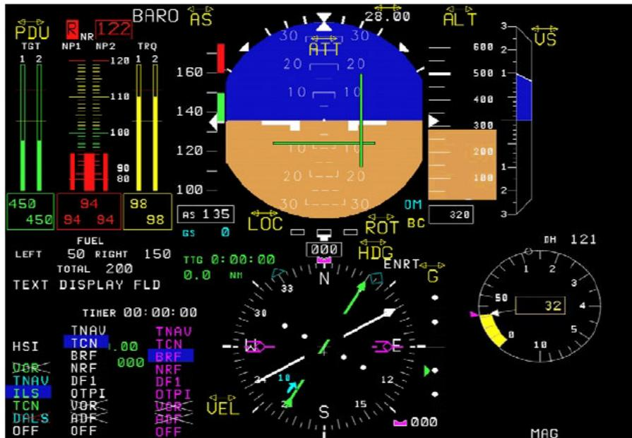
Fig. 6.1: Visual display of single take-off and landing flight.
