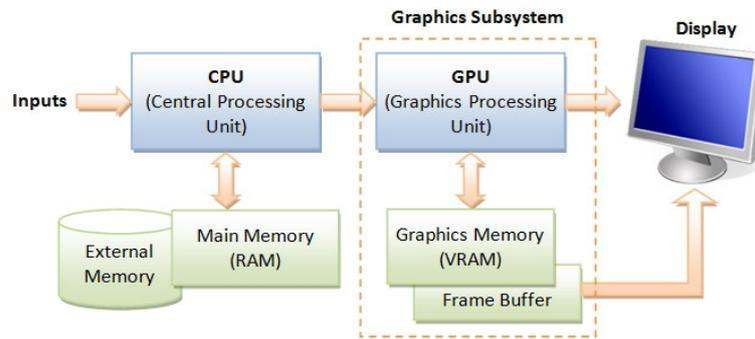
Fig. 2.1: How OpenGL works in a Windows environment.
