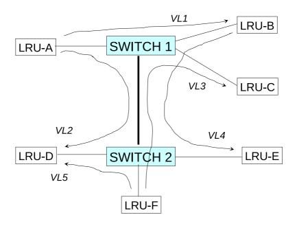
FIG. 5.3. Virtual Links between six LRU's in a system with two switches
