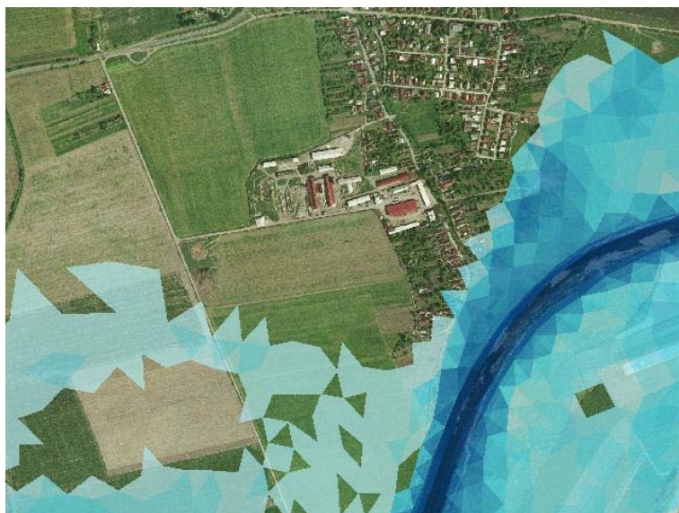
FIG. 3.1. Visualization of a flood simulation on the Váh river, Slovakia. The water poured out of the river bed and endangers the village. The intensity of colour shows the depth of the water. The colour turns into black in the river bed.
