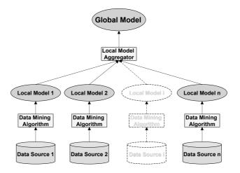
FIG. 3.1. General Distributed Data Mining Framework.
