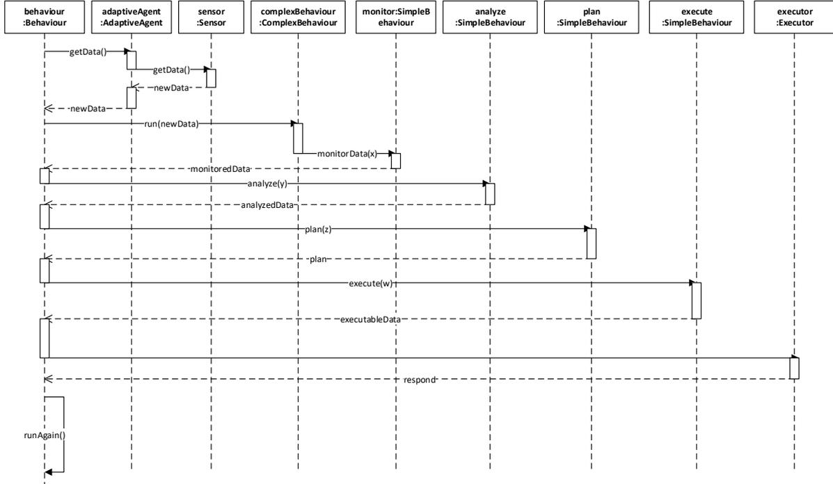
FIG. 3.8. Sequence Diagram of a simple MAPE loop
