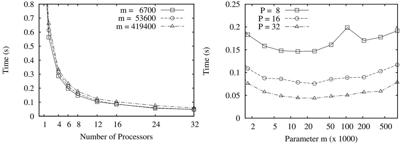
FIG. 6.3. For the prefix numbering problem, execution times plotted to the number of processors and to the parameter  $m$ . The input trees are from the same randomly generated tree divided with different parameter  $m$ .
