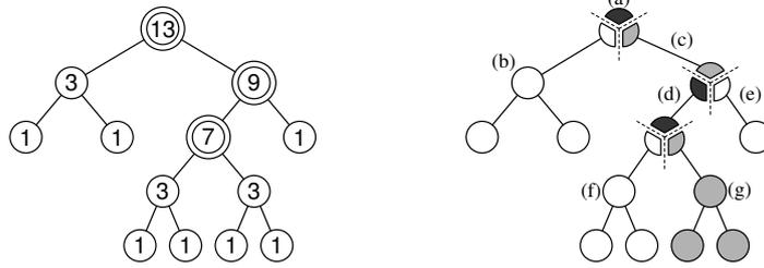
FIG. 3.1. An example of  $m$ -critical nodes and  $m$ -bridges. Left: In this binary tree, there are three 4-critical nodes denoted by the doubly-lined circles. The number in each node denotes the number of nodes in the subtree. Right: For the same tree there are seven 4-bridges, (a)–(g), each of which is a set of connected nodes.
