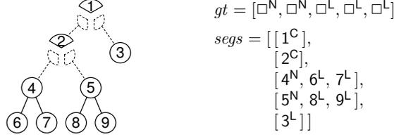
FIG. 3.2. Array representation of divided binary trees. Each local segment of  $segs$  is assigned to one of processors and is not shared. Labels L, N and C denote a leaf, a normal internal node, and an  $m$ -critical node, respectively. Each  $m$ -critical node is included in the parent segment.
