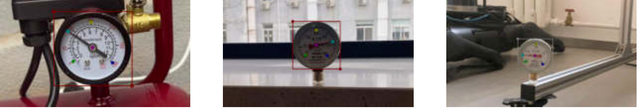
Fig. 3.1: Examples of pointer meter annotations. (a) Instrument A with a maximum range of 180 Lb/inš; (b) Instrument B with a maximum range of 0.6 MPa; (c) Instrument C with a maximum range of 1.6 MPa.
