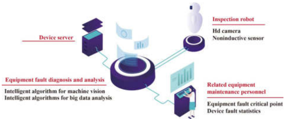
Fig. 3.1: Block diagram of fault detection system of intelligent inspection robot
