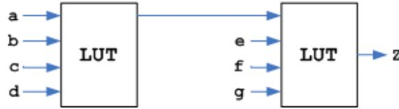
FIG. 2.1. Seven input bits to occupy two LUTs
