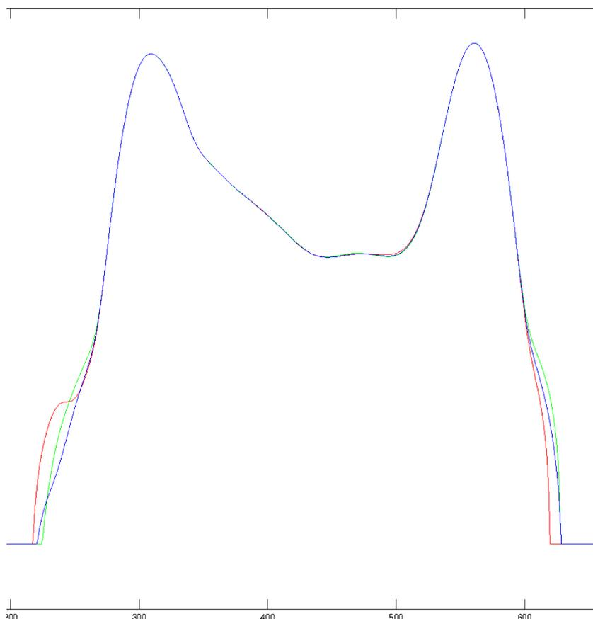
FIG. 5.3. Electron density obtained with MCM and Hybrid1 (Niederreiter) and Hybrid2 (Halton). The electric field is  $15[\text{kV/cm}]$  along to the nanowire.
