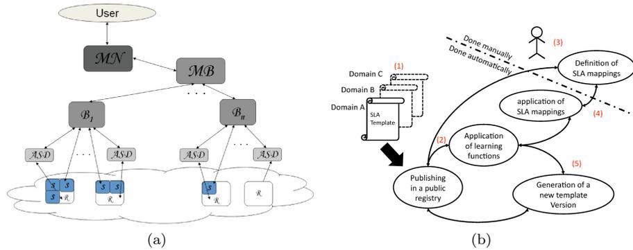
FIG. 7.3. (a) Architecture for the SLA-based Resource Virtualization [20] (b) Lifecycle of the SLA Template as used in [29]
