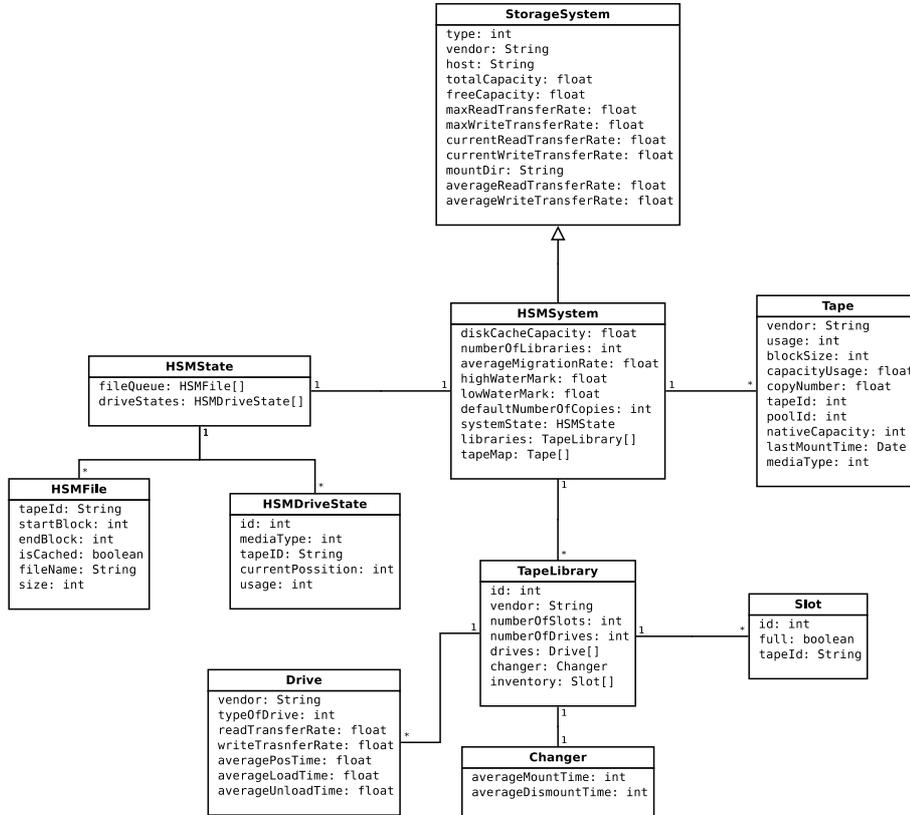
FIG. 3.1. CMSSM's class diagram for HSM system.
