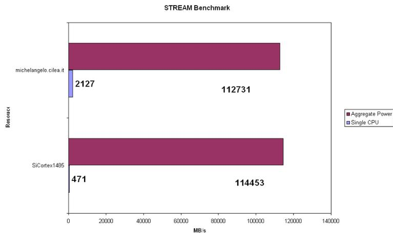
FIG. 5.2. Comparison between resources according to STREAM benchmark.
