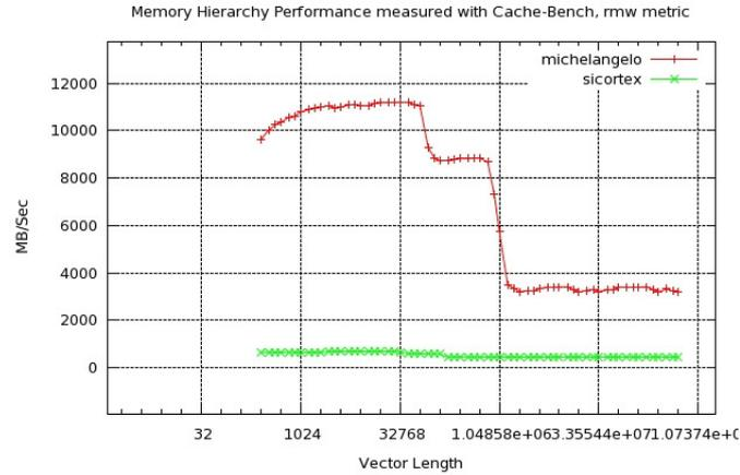
FIG. 5.3. Comparison between resources according to CacheBench.
