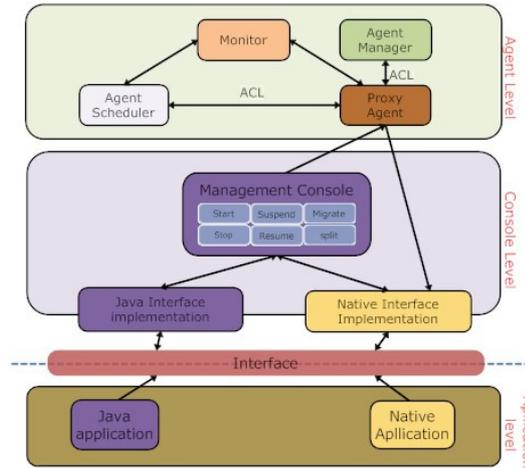
FIG. 4.1. *Software Architecture*
