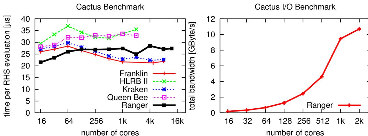
FIG. 3.1. **Left:** Weak scaling benchmark results of the McLachlan code on several current leadership HPC systems. This benchmark simulates a single black hole with nine levels of mesh refinement. The code scales well up to more than 12,000 cores of Ranger at TACC. **Right:** I/O benchmark on Ranger, showing the total I/O bandwidth vs. the number of cores. Cactus achieves a significant fraction of the maximum bandwidth already on 1,000 cores.
