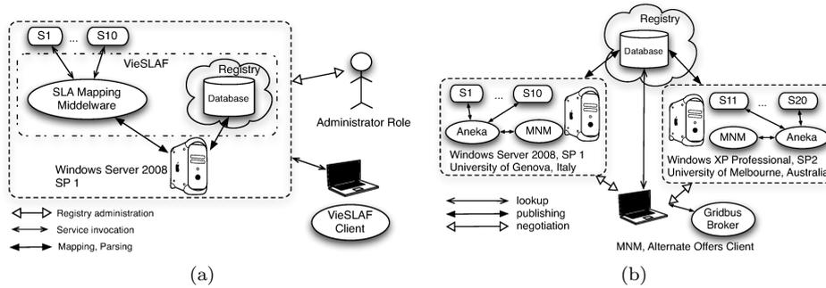
FIG. 7.1. *VieSLAF Testbed (a) for the evaluation of SLA mappings and (b) meta-negotiations*TABLE 7.1
