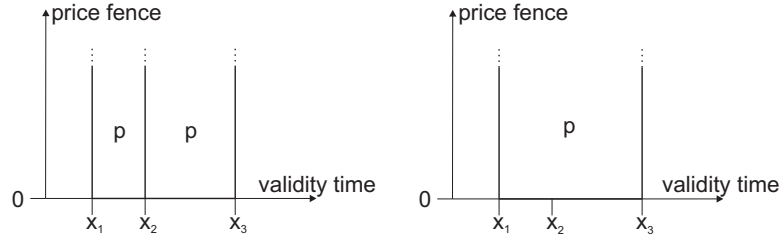
Fig. 5.1: Merging of horizontally adjacent PMCs (before and after).
