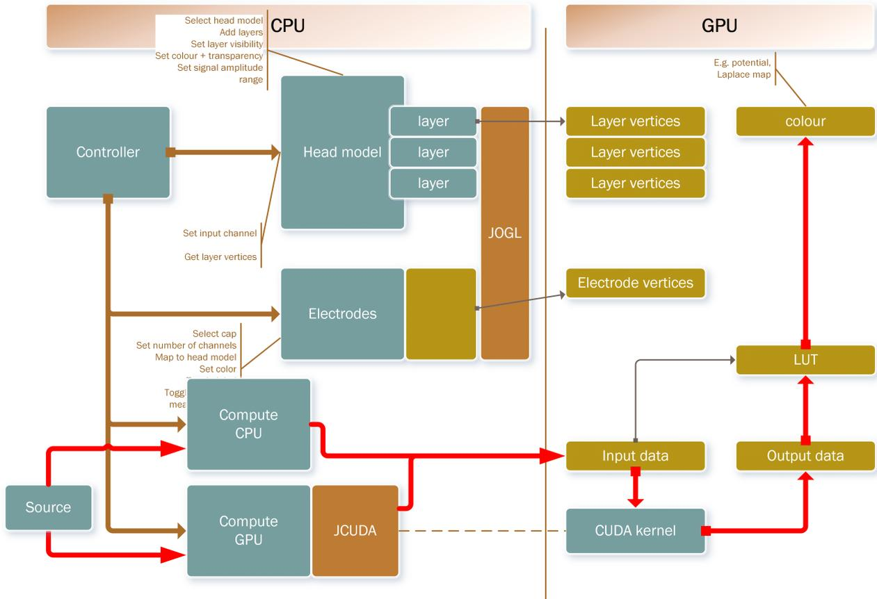
FIG. 4.2. The high-level view of the GPU stream architecture. Solid arrows indicate data movement, thick red arrow depicts live data update path (stream). Data copied to the GPU memory are available to both the OpenGL and the CUDA backend. Processing node may or may not have GPU implementation parts. Their number and order are not limited.
