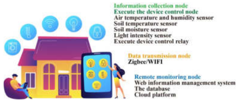
Fig. 3.1: Architecture diagram of smart agricultural greenhouse monitoring system based on Internet of Things technology
