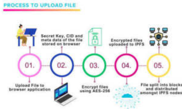
Fig. 6.1: Process diagram to upload the encrypted file using the proposed framework
