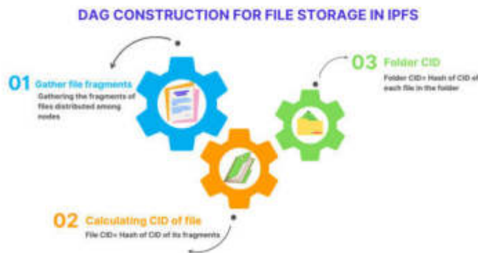
Fig. 4.2: DAG construction for file storage in IPFS
