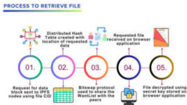
Fig. 6.2: Process diagram to download and decrypt the file from the proposed framework
