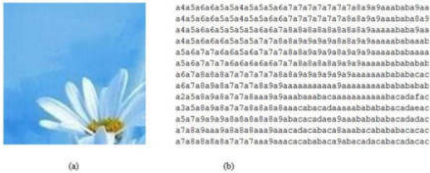
Fig. 4.1: a) Source image of resolution 128x128 b) Image pixels as hexadecimal values in text file
