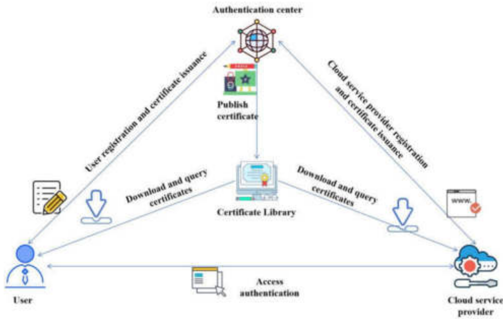
Fig. 3.1: Basic structure of PKI system
