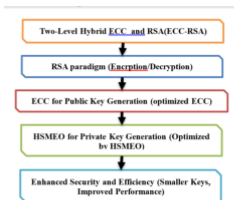
Fig. 3.3: Two-Level Hybrid ECC and RSA (ECC-RSA) Model
