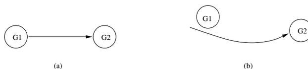
FIG. 4.4. (a) Connected dataflow graphs and (b) Non-connected Lazy graphs. In scenario (a),  $G_2$  needs to wait for  $G_1$ . This scenario is applicable if the Operand port in  $G_2$  is strict. In scenario (b),  $G_2$  can start before  $G_1$  executes. The Operand port in  $G_2$  is non-strict in this scenario. In the first case,  $G_1$  is the Predecessor graph and  $G_2$  is the Successor graph. In the second case (b),  $G_1$  becomes Successor and  $G_2$  becomes Predecessor.
